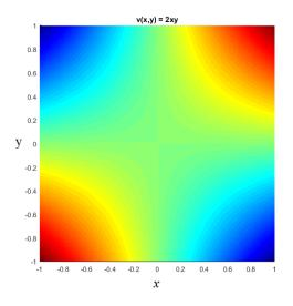
[X Y] = meshgrid(-1:0.01:1);  $U = X \cdot ^{2} - Y \cdot ^{2};$  $V = 2^{*}X.^{*}Y;$ subplot(121); surf(X,Y,U, 'EdgeColor', 'none'); view(2); title('u(x,y) =  $x^{2}-y^{2}$ '); subplot(122); surf(X,Y,V, 'EdgeColor', 'none'); view(2); title('u(x,y) = 2xy'); colormap jet;
